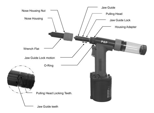
For optimum tool performance, Front-End maintenance should be performed regularly as per the "Preventative Maintenance Schedule".
